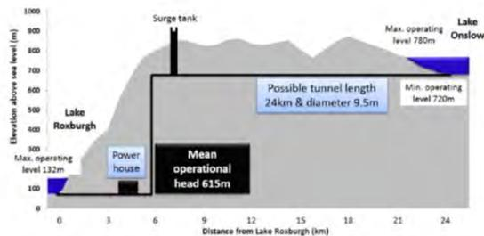
Figure 3.12 Cross section of the simulated Onslow PHES.
