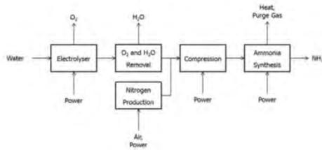
Figure 2.2: Block Diagram of Power to Ammonia
