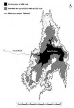
Figure 3.10 The hypothetical Onslow basin at 780 msl as the maximum extent of development and 720 msl as the minimum operational level.
