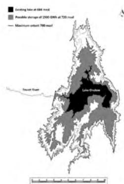
Figure 3.10 The hypothetical Onslow basin at 780 msl as the maximum extent of development and 720 msl as the minimum operational level.
