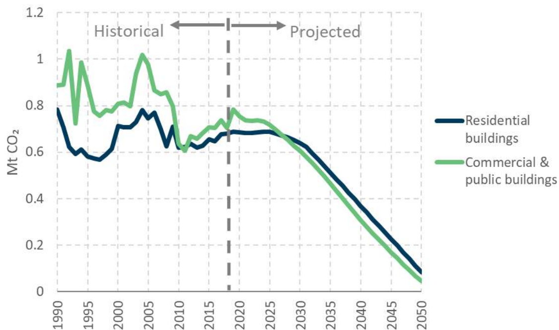
Figure 8.19: Historical and projected emissions from fossil fuel combustion in buildings in the Tailwinds scenario
